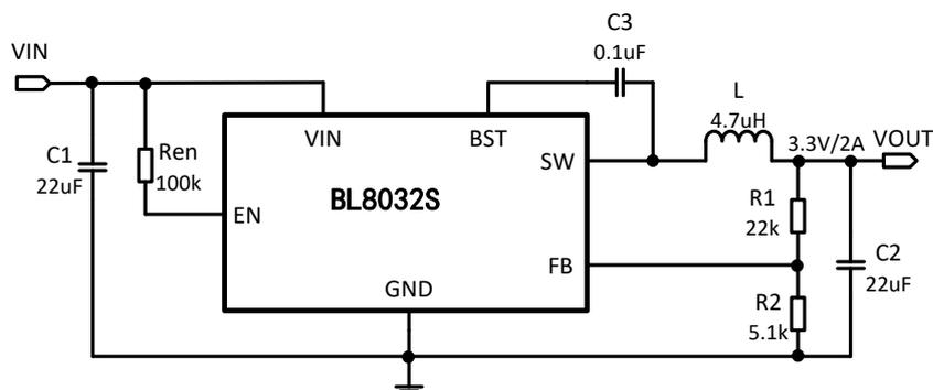
**Note:** 1) C1 and C2 recommended using 22uF ceramic capacitors. If the electrolytic capacitor is used, it is recommended that the ceramic capacitor in parallel with a capacitance value of 0.1uF or more.
